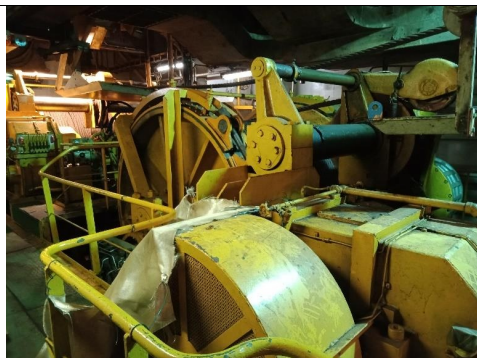
7) Anchor mooring winch at below main deck.
