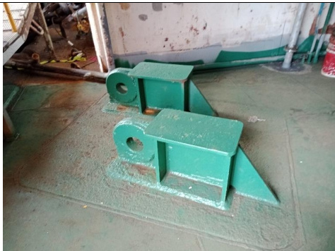
25) Main and emergency towing pad eye at forward.
