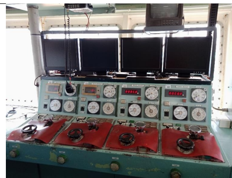
6) Anchor mooring winch console station at control tower.
