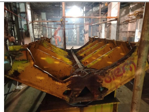
12) Pipeline guide in the firing line.
