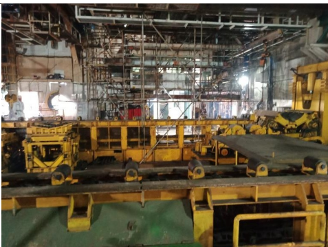
9) Pipeline lining up station.
