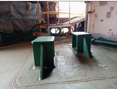
26) Towing pad eye and fairlead.
