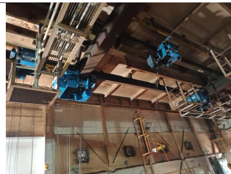
10) Overhead crane at pipeline lining up station.
