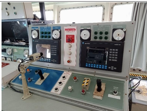
15) Pipelay tensioner console at control tower.
